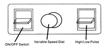
**On/Off Switch** – Up for On, Down for Off
