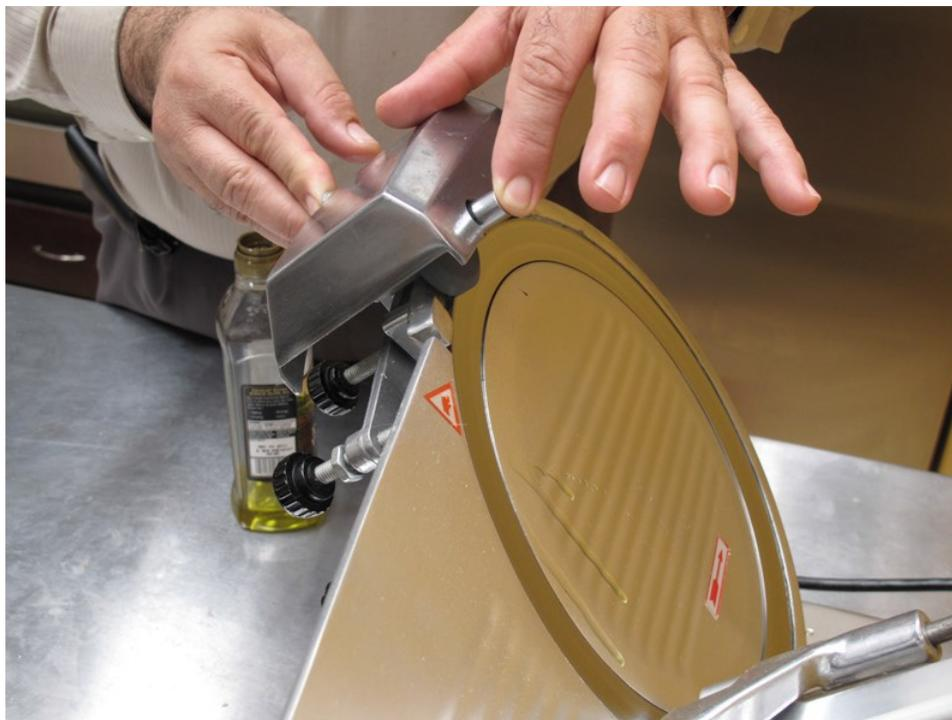
7. Push the button on the back of the sharpener to begin to sharpen the rear of the blade.
