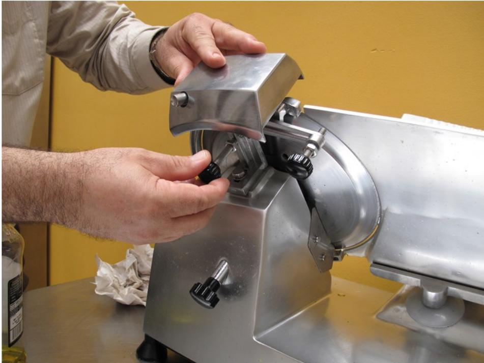
9. Inspect your blade and clean it before usage. Be sure to clean off all the metal pieces and leftover oil. After your first few slices of meat with the sharpened machine, inspect the sliced product for metal shavings and discard if necessary.
