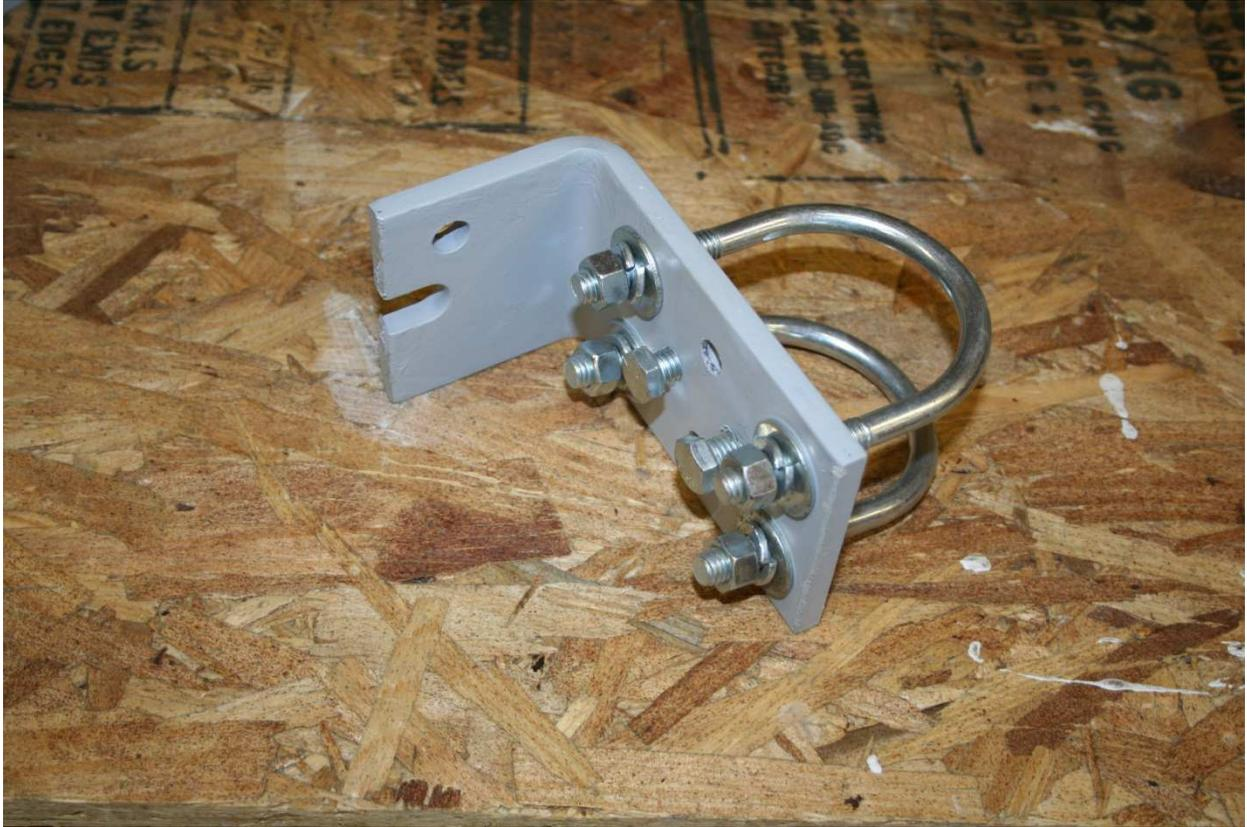
One of two bracket assemblies with holes drilled to the same distance from the gate as the original black bracket.
