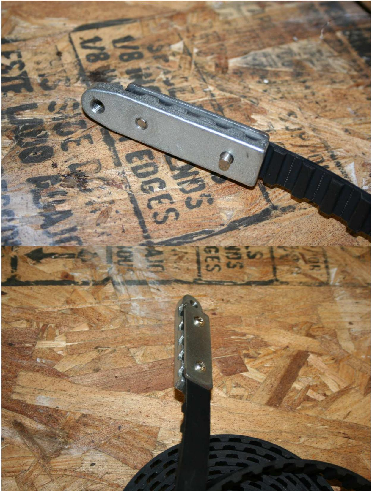
These are photos of the drive belt with mounting attachments at each end.
