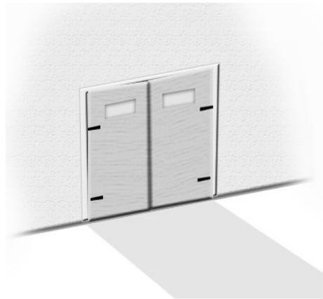
**Both doors are programmed simultaneously. Both leafs will move together through the same programming sequence. There is a slight starting delay on the slave side.**
